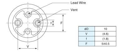
Products of vent on rubber type, please make clearance about 1mm minimum between rubber and board. If it is difficult to make clearance 1mm minimum between rubber and board, please arrange gas escaping hole on the board (same position and 40% minimum diameter from the vent).
