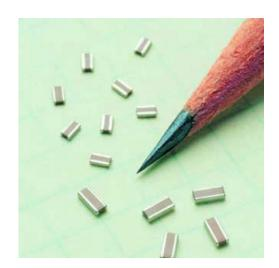
LICC capacitors are specially designed to exhibit lower inductance by altering the aspect ratio of the terminations. The smaller current loop length results in Equivalent Series Inductance (ESL) that is typically 60% lower then standard MLCs of the same size. This ESL improvement is extremely advantageous in the high frequency power decoupling of high speed digital MPU, FPGA, DSP, etc..
